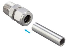
Insert well prepared tubing into VEE-LOK two ferrule tube fittings until tubing end is firmly seated on the body shoulder.
