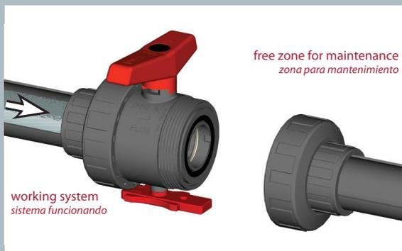
With the threaded seal-carrier, we are able to isolate the pump zone for maintenance. The thread is supporting the pressure of the system.
